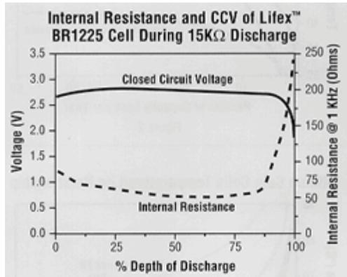
Figure 2. Closed Circuit Voltage and Internal Resistance Over Discharge.
